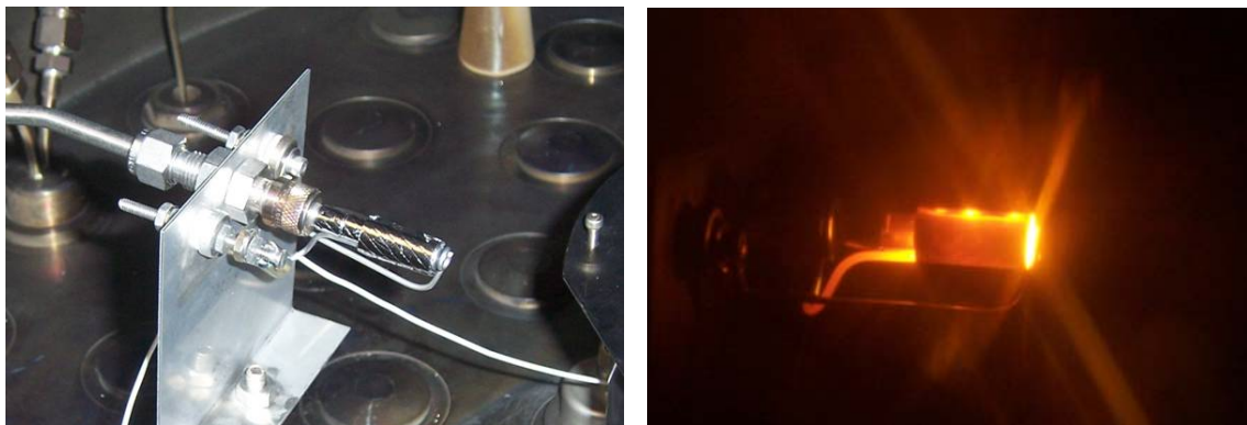
Figure 1 Hollow cathode test setup. The toroidal electrode located immediately downstream of the cathode orifice plate is used to measure emission current from the cathode during testing without gas flow and to initiate and sustain a discharge during testing with gas. The visual glow of the cathode corresponds to a heater current setting of 7.0 A and suggests that a significant fraction of heat loss from the cathode is due to radiation. Radiation shielding comprised of thin tantalum foil is wrapped around the cathode heater, which reduces radiation losses.
