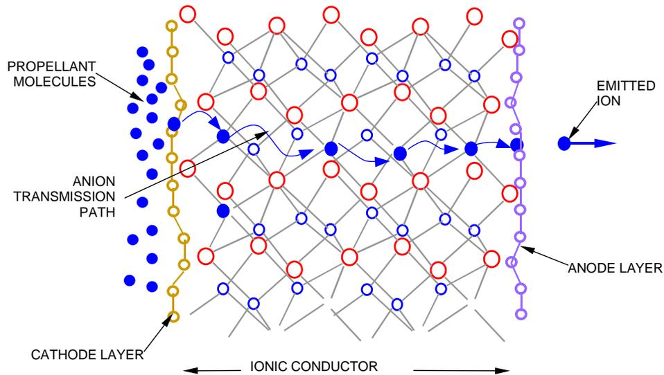
Fig. 2 Membrane Process Diagram for Anion Transmission
