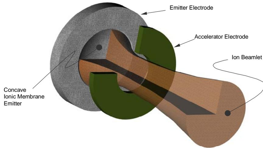
Fig. 3 The Emissive Membrane Ion Thruster Concept
