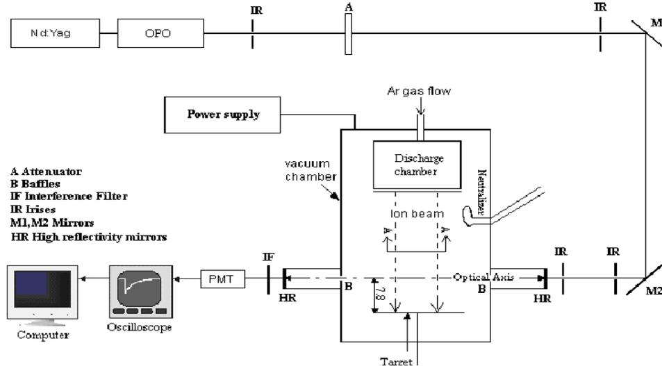
**Figure 2. Schematic diagram of CRDS set-up. An ion source and target are housed within a vacuum chamber. Sputtered species are created as the ion beam bombards the target. The plume of the sputtered species is intersected by the optical axis of the high-finesse ring-down cavity. An OPO laser system is used as the light source, and a photomultiplier tube (PMT) detects the light exiting the cavity.**
