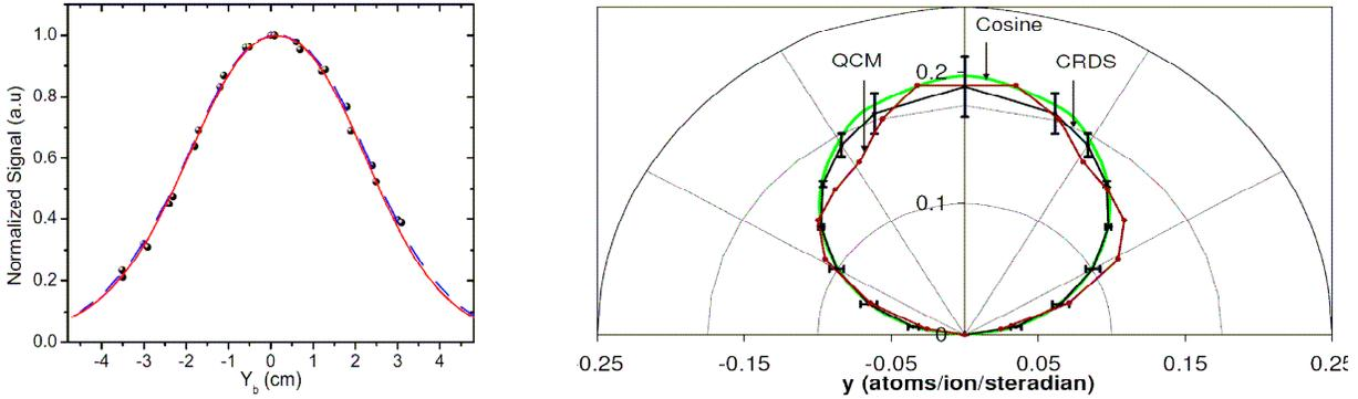
**Figure 7. Differential sputter yield measurement of sputtered tantalum. Left: CRDS spatial profile. Symbols – CRDS data, Red solid line – model fit to CRDS data ( $a=0.0$ ), Blue dashed line – modeled profile based on QCM data. Right: Polar plot of differential sputter yield profiles. Black line – modeled profile from fit to CRDS data ( $a=0.0$ ), Brown line – QCM data, Green line – diffuse profile (see text).**
