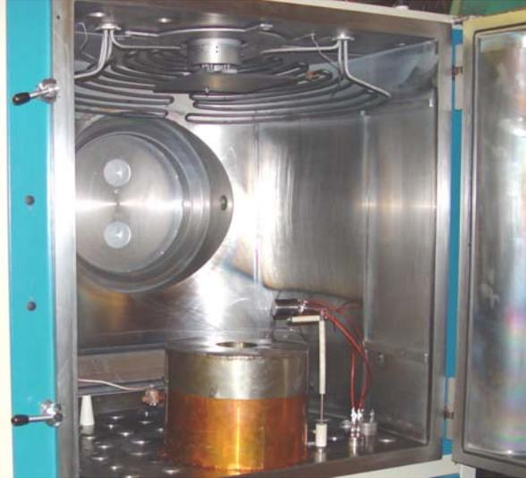
Figure 1: High voltage sub-scale ion optics testing facility
