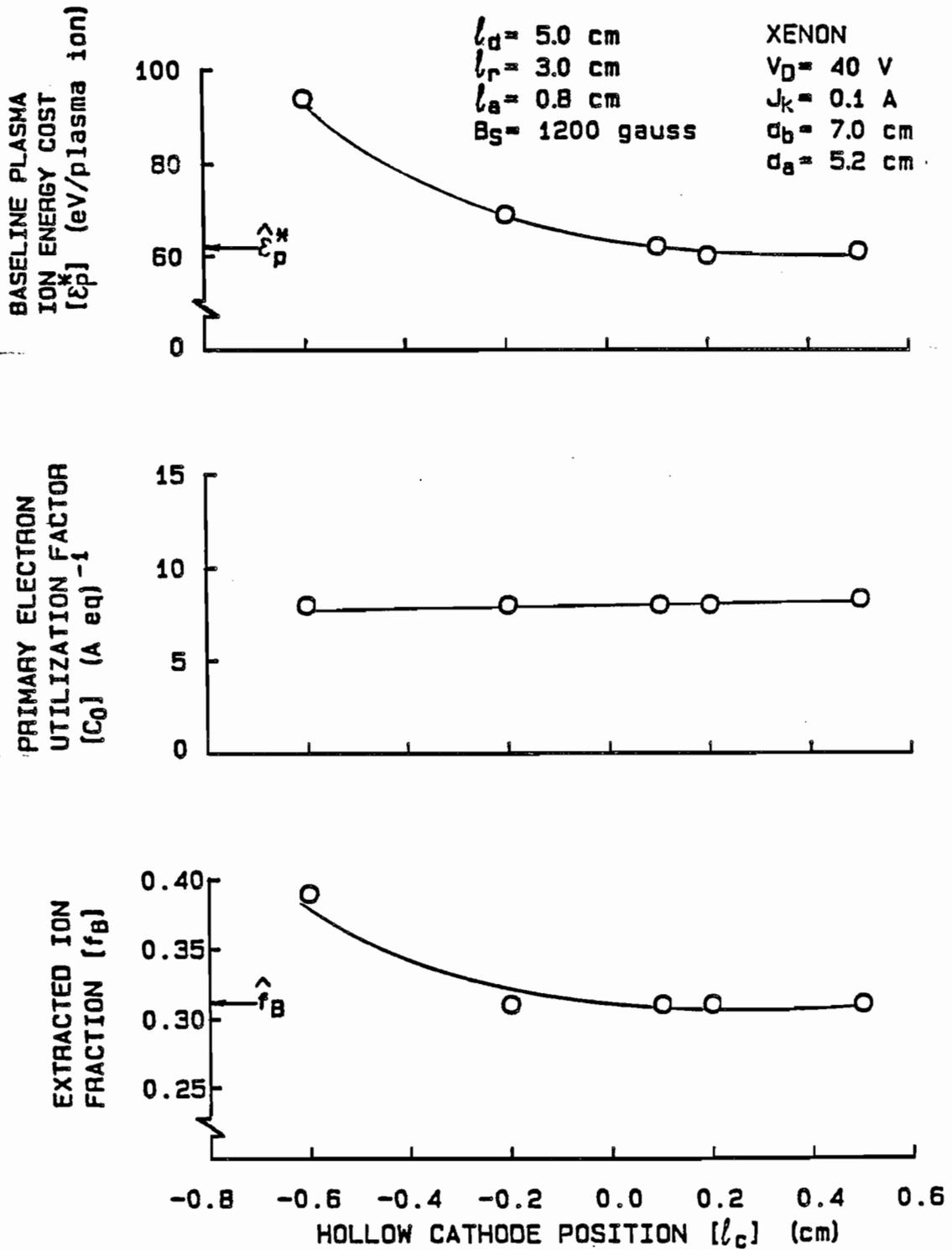
Fig. 13 Effect of Centerline Hollow Cathode Axial Position on Discharge Chamber Performance Parameters
