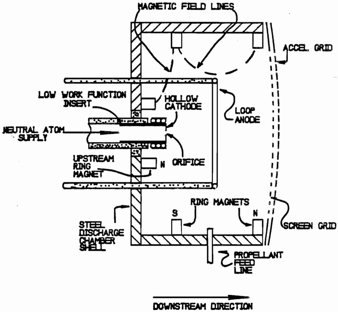
Fig. 1 Generic Discharge Chamber
