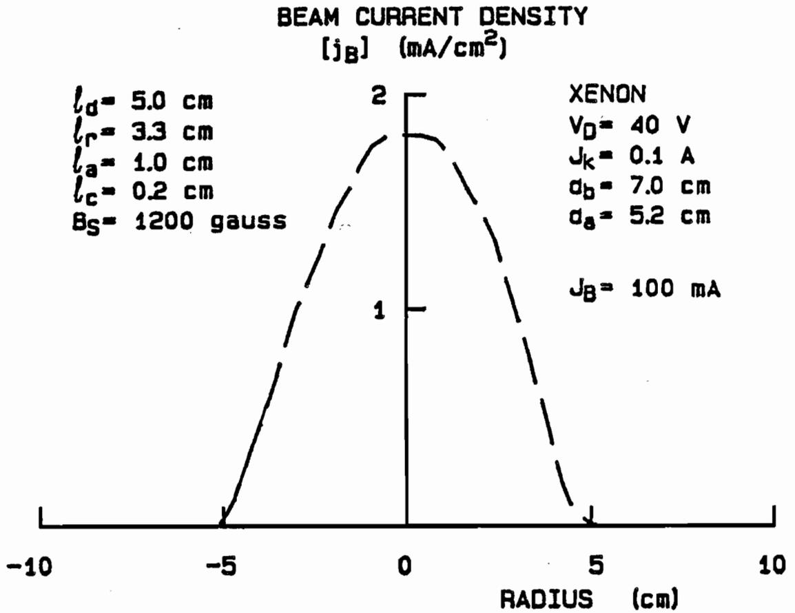
Fig. 4 Typical Beam Current Density Profile
