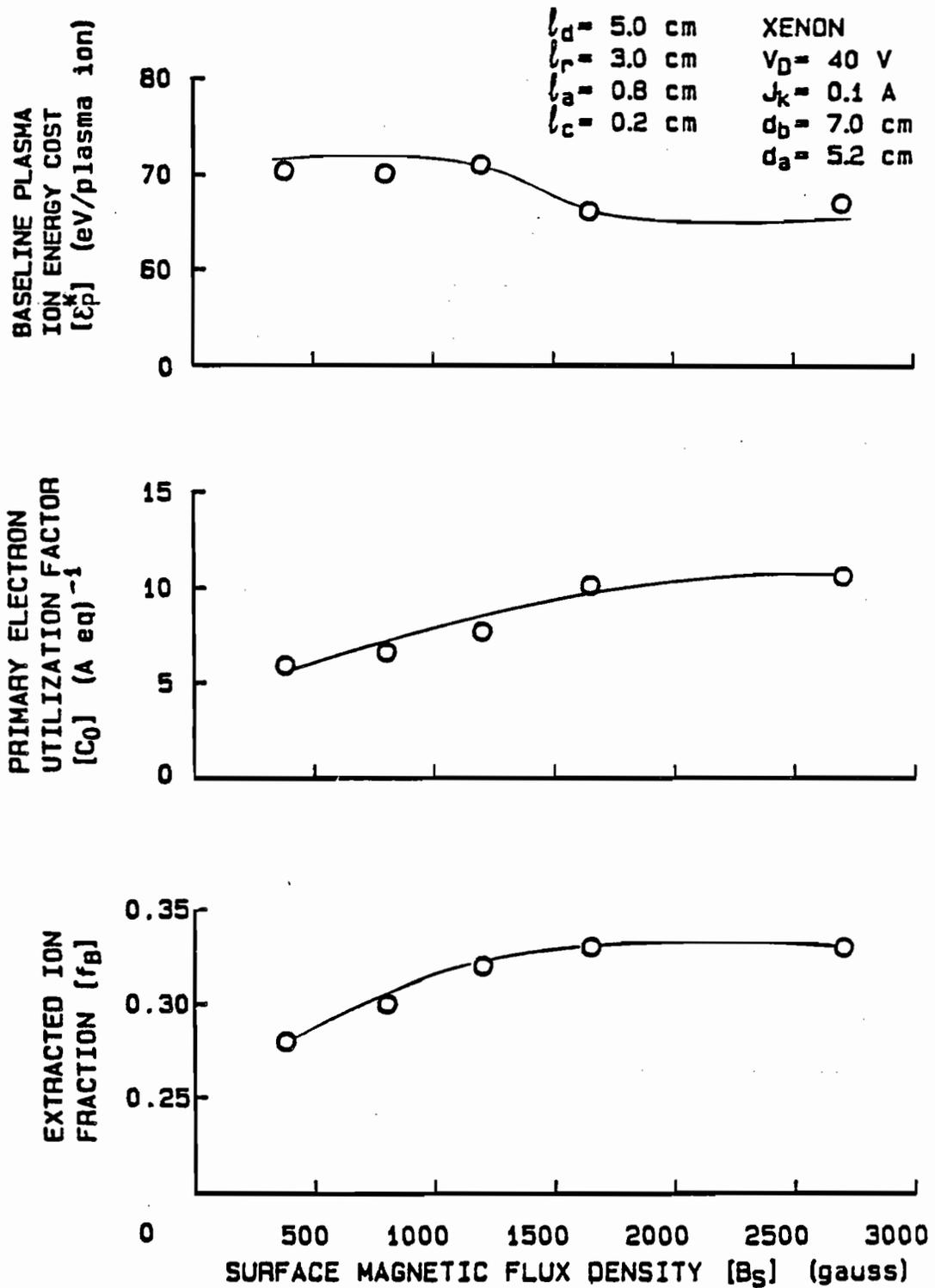
Fig. 17 Effect of Magnet Strength on Discharge Chamber Performance Parameters
