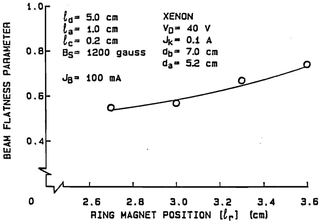
Fig. 22 Effect of Ring Magnet Position on Beam Flatness Parameter
