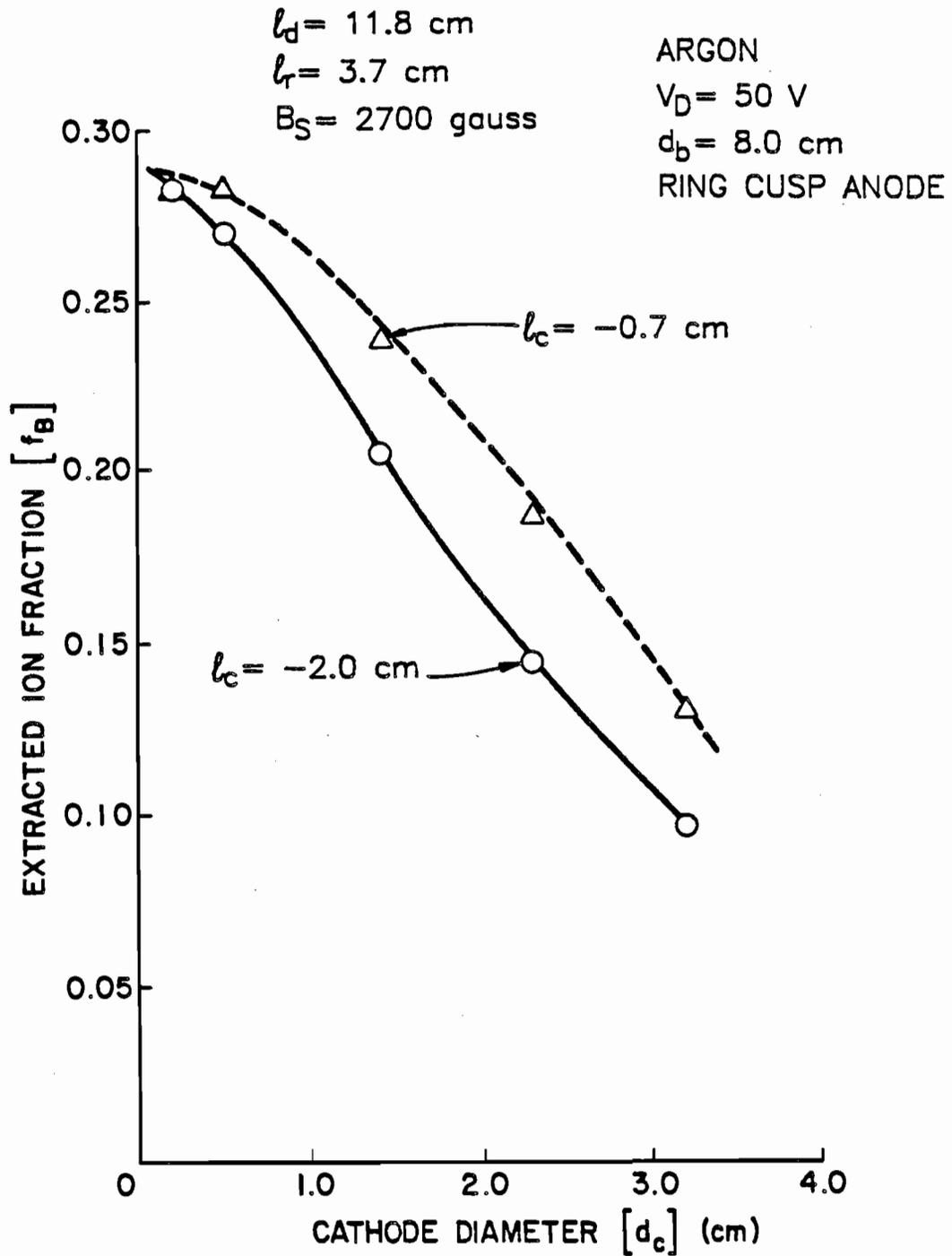
Fig. 11 Effects of Upstream Filament Cathode Diameter and Position on Extracted Ion Fraction
