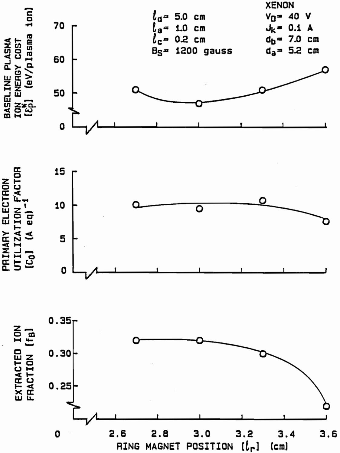
Fig. 20 Effect of Ring Magnet Position on Discharge Chamber Performance Parameters
