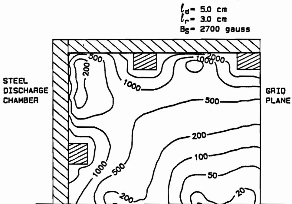
Fig. 19b Magnetic Flux Density Contour Map
