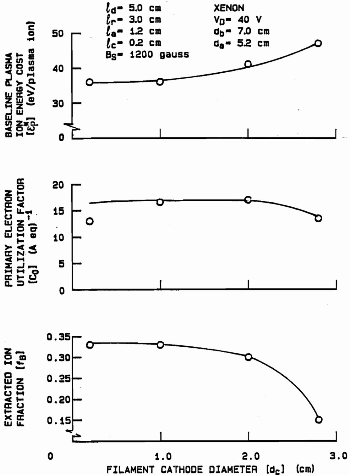
Fig. 15 Effects of Downstream Filament Cathode Diameter on Discharge Chamber Performance Parameters
