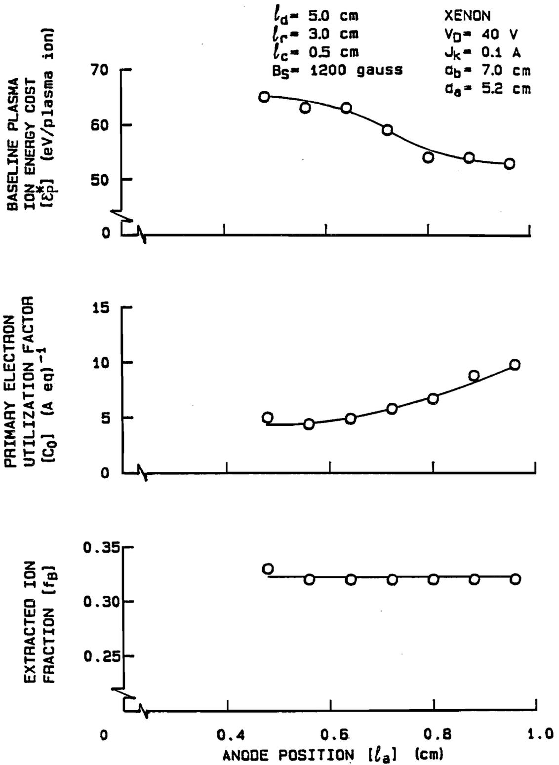
Fig. 16 Effect of Anode Position on Discharge Chamber Performance Parameters
