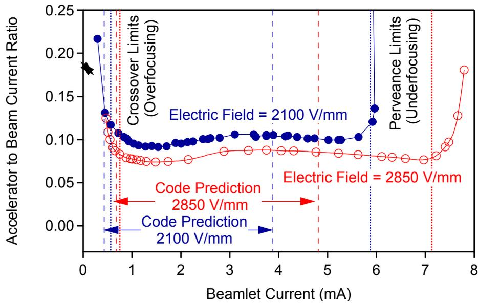
**FIGURE 3.** CETDP grid performance measured in subscale gridlet tests and predicted by the design codes.
