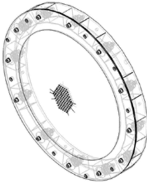
**FIGURE 5.** Ion optics assembly for the CBIO grids showing the screen grid bonded to a strong, lightweight carbon-carbon box structure.
