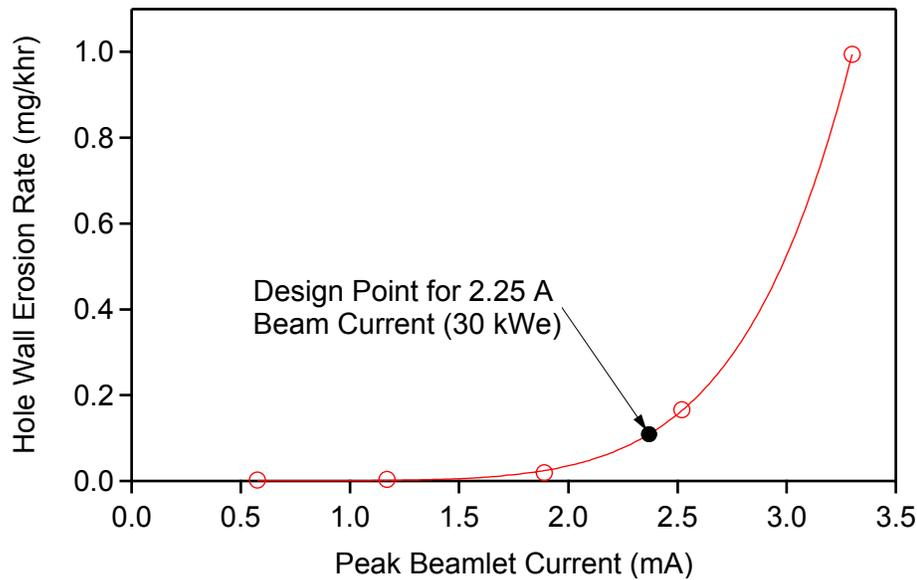
**FIGURE 4.** Hole wall erosion rates in the CETDP grid design increase dramatically as the beamlet current approaches the perveance limit.
