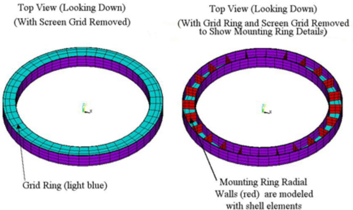
**FIGURE 6.** Mounting structure used in dynamic loads analysis of CETDP grids.
