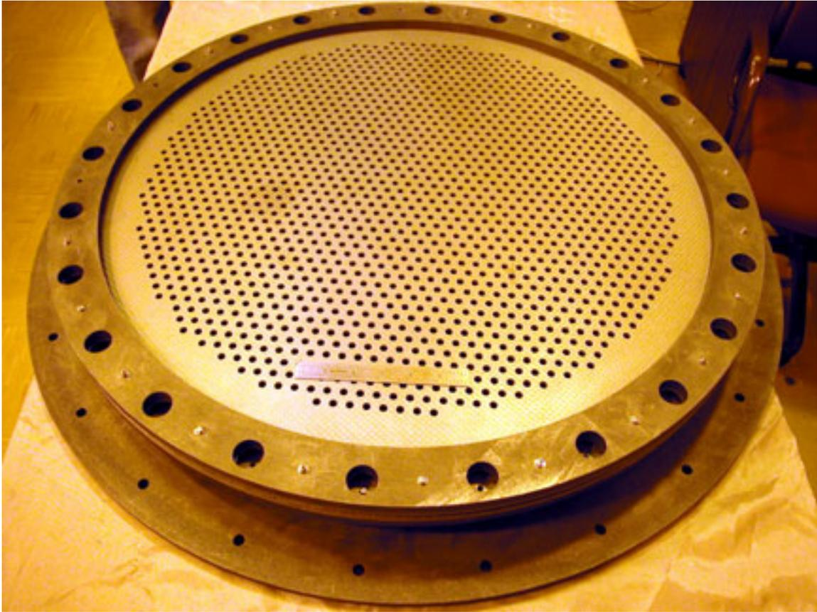
**FIGURE 7.** 75-cm diameter carbon-carbon grids designed to operate at 14000 s.
