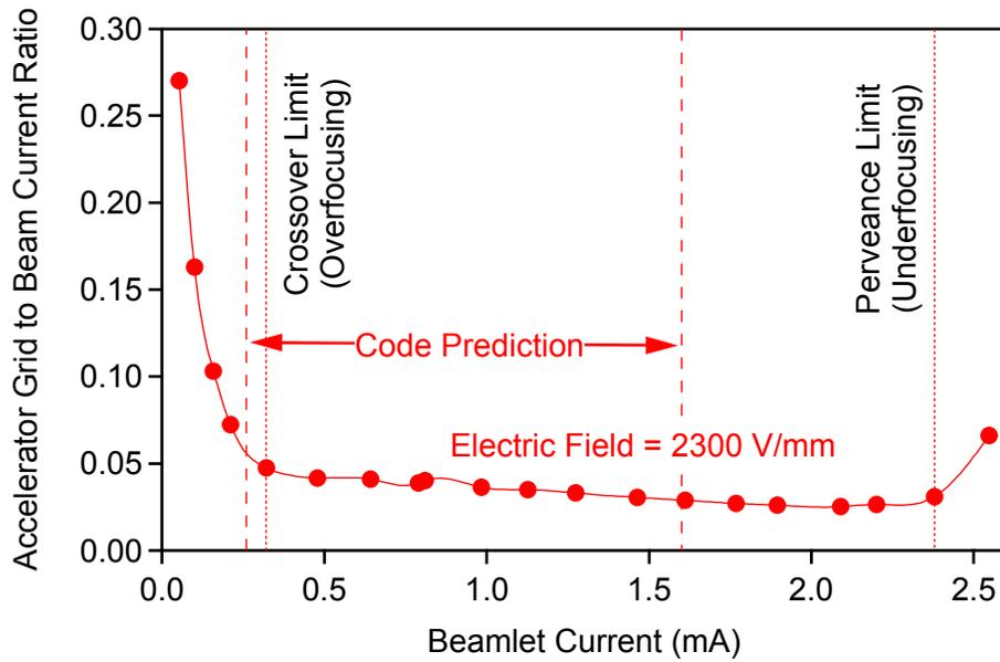
**FIGURE 2.** NEXIS grid performance measured in subscale gridlet tests and predicted by the design codes.
