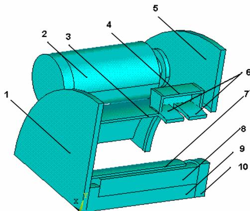
**Fig. 1. Hall thruster magnetic system.**
