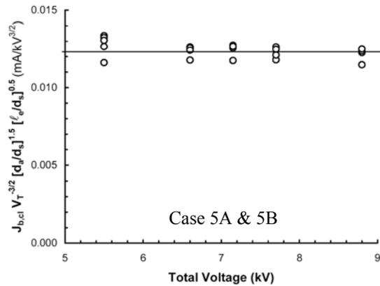
Fig. 8c. Normalization of crossover limit data using experimentally measured sensitivities. (See Table 2)
