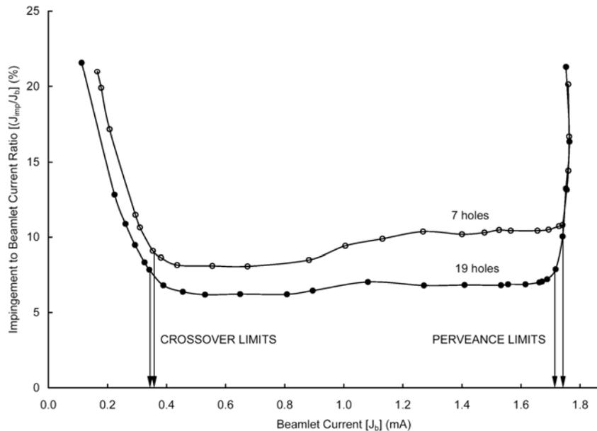
Fig. 3. Effect of changing the number of holes on impingement limit data. (Case A,  $V_N = 6.5$  kV.)
