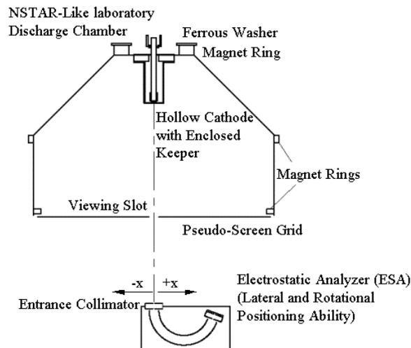
Fig. 1a Schematic of prototype NSTAR discharge chamber.
