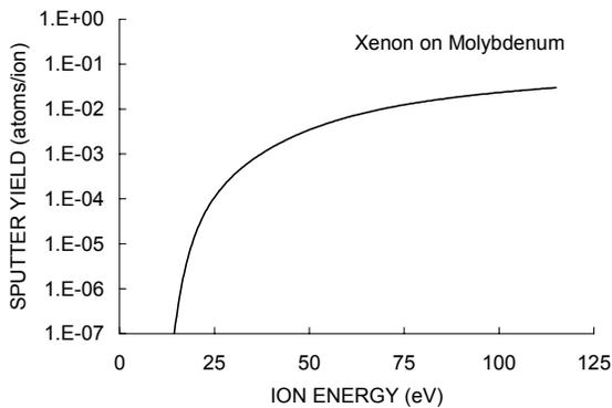
Fig. 4c) Sputter yield data for xenon on molybdenum.
