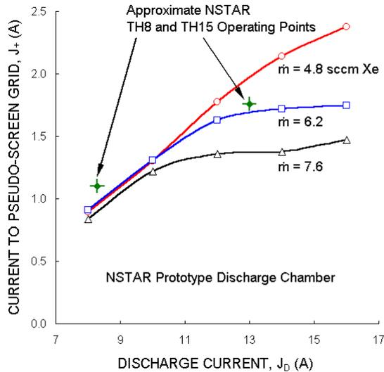
Fig. 2b NSTAR-like discharge chamber beam current comparison.
