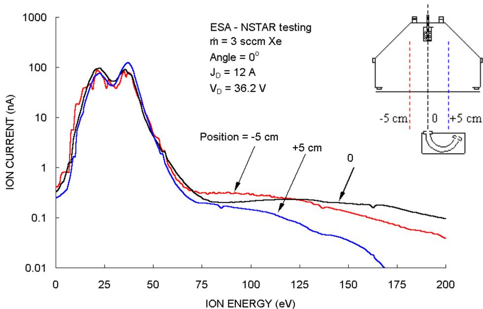
Fig. 6 ESA measurements at positions of -5, 0, and +5 cm.
