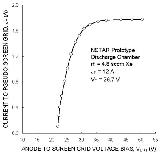
Fig 2a Saturation current to the pseudo-screen grid.
