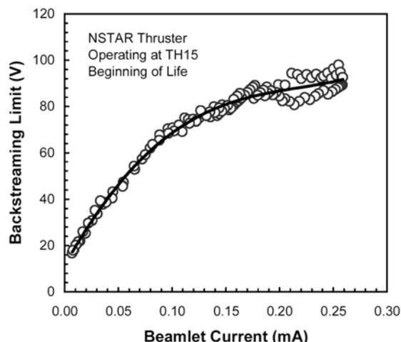
Fig. 8 Analytical prediction of the backstreaming limit for the NSTAR thruster as a function of beamlet current calculated using measured beamlet diameters from Soulas and Rawlin (1999).
