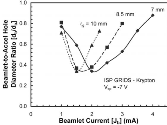
Fig. 5 Beamlet diameter calculations for the ISP grids.
