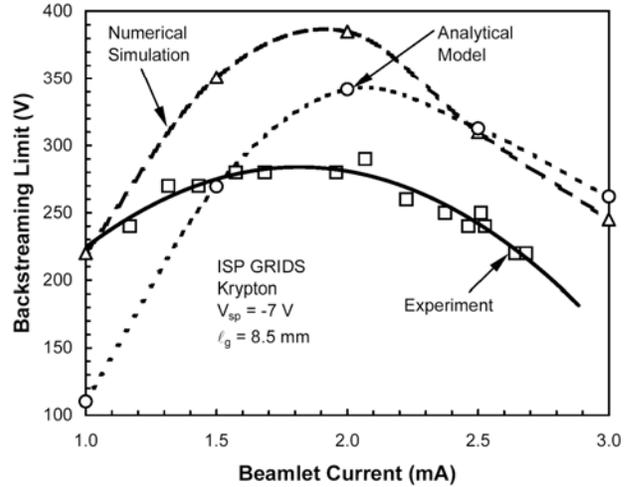
Fig. 6b Backstreaming comparisons at a spacing of 8.5 mm.
