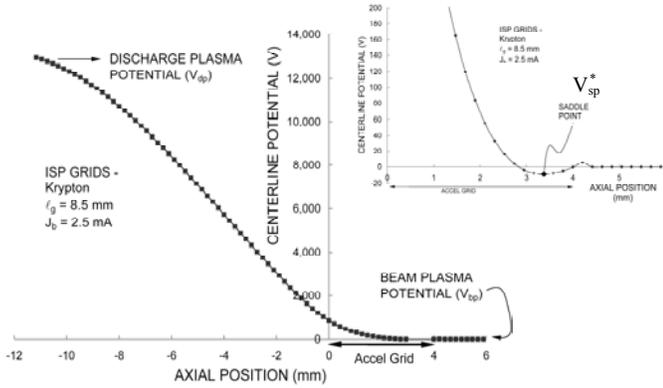
Fig. 1 Typical high Isp grid set potential profiles at the point where backstreaming onset will occur. Inset shows exploded view near the accel grid location.
