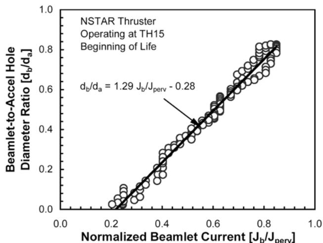
Fig. 7 Variation in NSTAR beamlet diameter as a function of beamlet current (from Soulas and Rawlins, 1999)
