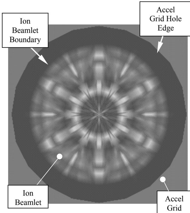
Fig. 3 Typical ion density pattern in an accel hole.
