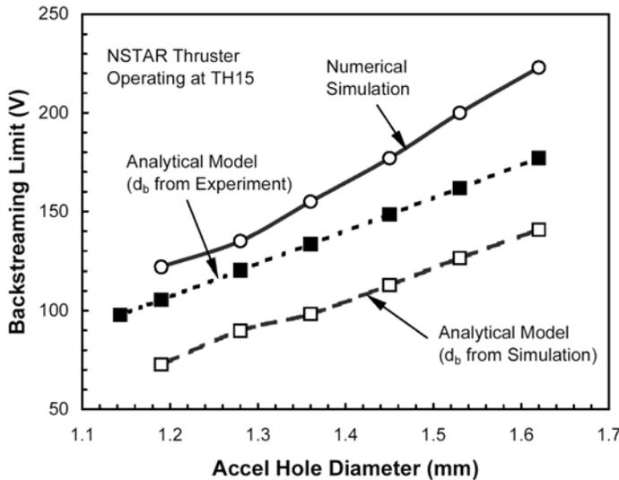
Fig. 9 Comparison of backstreaming limit variation with  $d_a$ .
