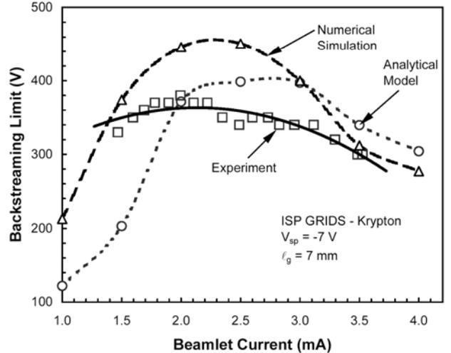
Fig. 6c Backstreaming comparisons at a spacing of 7 mm.
