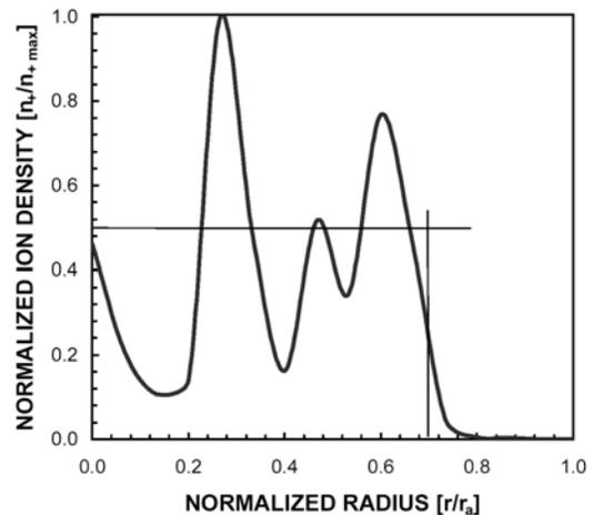
Fig. 4 Typical azimuthally averaged radial ion density profile in an accel hole.
