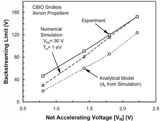
Fig. 10 Comparison of backstreaming limit variation with  $V_N$ .
