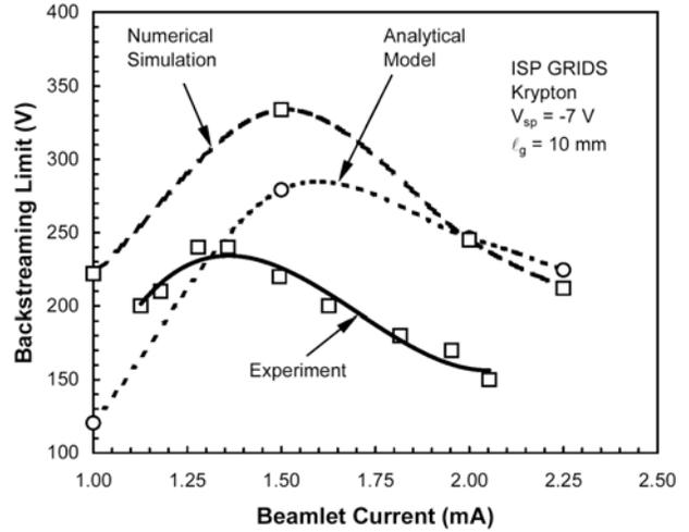
Fig. 6a Backstreaming comparisons at a spacing of 10 mm.
