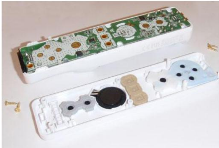
Figure 3- After the two pieces of the case pulled apart (Note: that in this picture, one of the cases is flipped)
